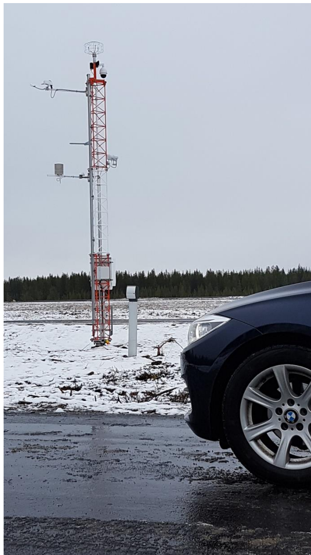
Figure 3. Road weather station in the Sod5G test track.
