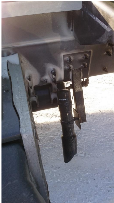
Figure 6. Teconer RCM411 and RTS411 instruments (used both in Intelligent Arctic Trucks and Sod5G mobile friction measurements).
